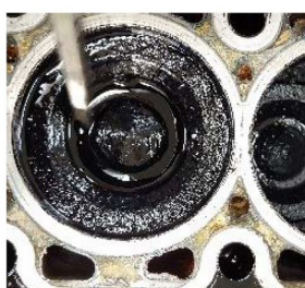
< Engine oil in combustion chamber >
